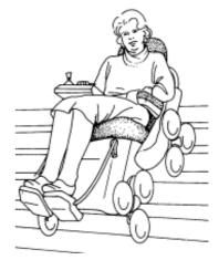
Although the angle of the seat unit adjusts on the stairway to keep the seat horizontal, users must have good trunk
