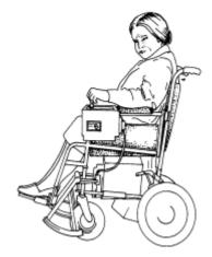
A wheelchair without kerb climbers may be able to negotiate a small raise of up to 5cm. With the addition of kerb climbing devices, a higher kerb of at least 10cm can be negotiated. Check with suppliers the recommended maximum height for each wheelchair and the technique you should use to climb and descend kerbs safely.
