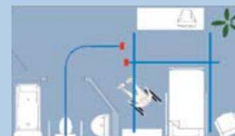
Gate allows the lift to transit in and out from a single track system into the X-Y system.
