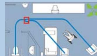
Exchanger functions like a junction on the road. It allows the lift access from one care area to separate care areas.
